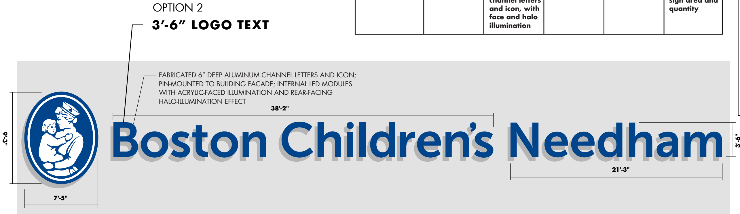
1 Detail Elevation scale: 3/16" = 1'-0"
