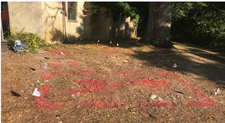
GPR data shows the peak of the tank, approximately 1 1/2' below the surface.
