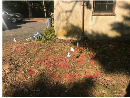
Picture 2: secondary view of “possible” tank location. The white flags represent vent piping that can be seen on the wall. Pipe depth was between 1’ – 1 ½’ deep.
