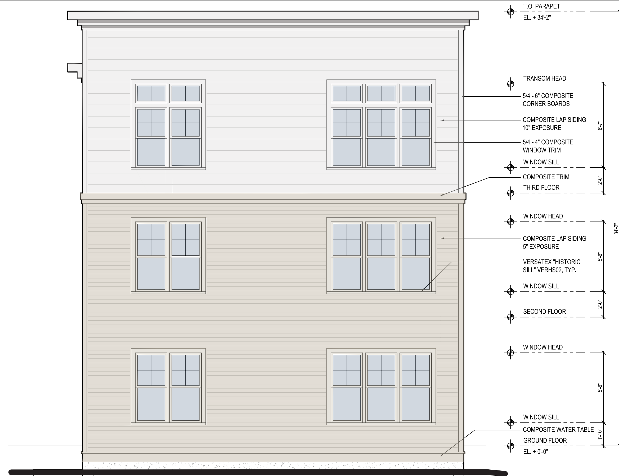
1 REAR ELEVATION SCALE: 1/4" = 1'-0"
