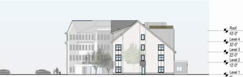
Phase 1 South Elevation 1/32" = 1'-0"
