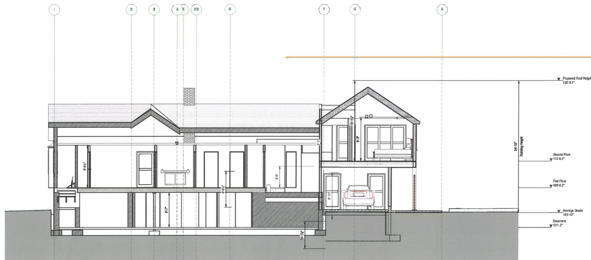
1 LONGITUDINAL SECTION : ENTRY ; LIVING ROOM; GARAGE SCALE: 1/4" = 1'-0"
