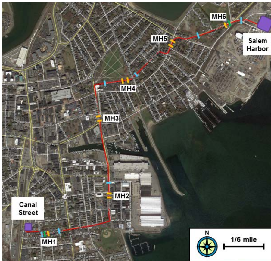
Figure C-1. Aerial view of transmission line route including terminus points, manhole locations and measurement transects. The color of measurement transects corresponds to those used in Figure 1 in the body of the report.
